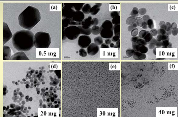
Figure 1. Transmission electronographs of Au nano-particles prepared at auxiliary surfactant of (a) 0.5, (b) 1, (c) 10, (d) 20, (e) 30 and (f) 40 mg; scale bar represents 20 nm.
