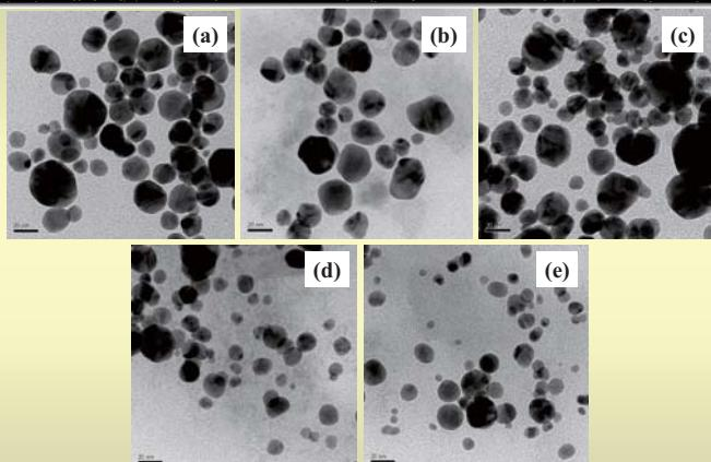
Figure. TEM image of Au nano-particle at CTABr of (a) 0.08, (b) 0.1, (c) 0.12, (d) 0.14 and (e) 0.16 M; Scale bar of image is 20 nm. Laser wavelength at 1064 nm.
